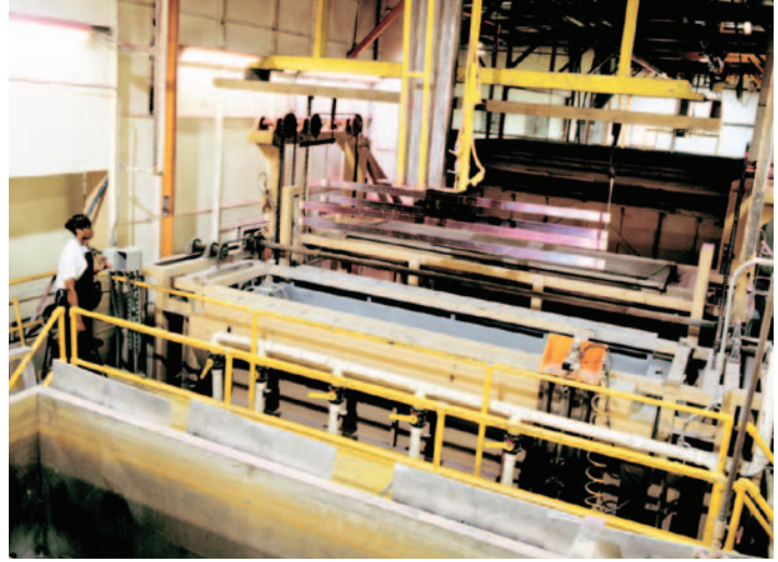
The preheated copper bars are shown prior to immersion in the epoxy powder.
