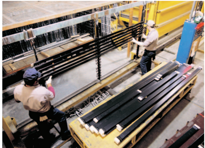
All phase and neutral bars receive a coating of Class B, 130°C, epoxy insulation applied by a fluidized bed process. The copper feeder bars are shown being withdrawn from the bed and sent to a cure oven.
