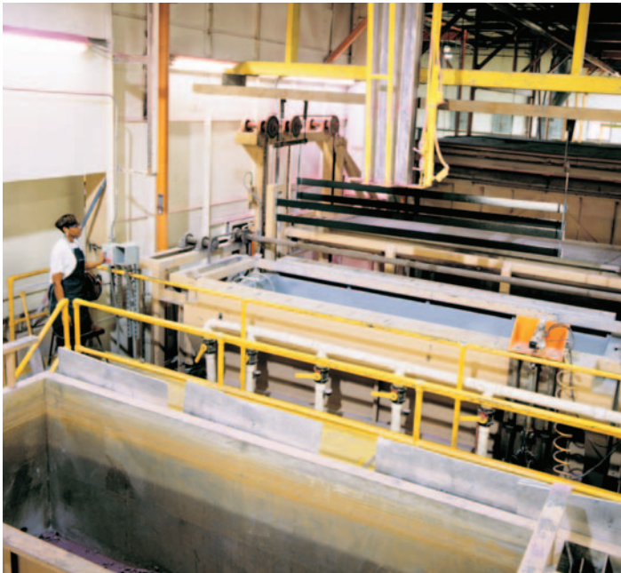
All phase and neutral bars receive a coating of Class B, 130°C, epoxy insulation applied by a fluidized bed process. The copper feeder bars are shown being withdrawn from the bed and sent to a cure oven.
