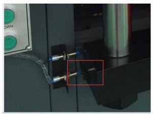
(The blank steel strip is the sensor, the two blue part is the limit switches, they are on bottom left of the punching cylinder)
