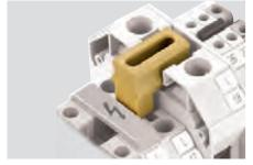
For the W-Series, power is supplied via standard terminals in conjunction with a special cross-connection, which directly connects terminals for larger and smaller cross-sections (the picture shows WDU 35 on WDU 4).
