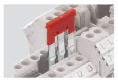
A screw-in and a plug-in cross-connection system is available for Weidmüller screw terminals. The plug-in **cross-connection (ZQV)** for screw terminals is unique. It enables considerable reductions in assembly times. The plug-in cross-connections can be used for nearly all W-Series terminals in the cross-section ranges 2.5 and 4 mm<sup>2</sup>.
