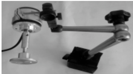
Diagram for installation of 1mm linear sensor (oil switch)
